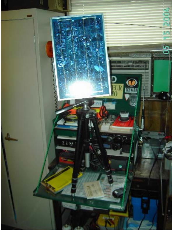
A 10 watt solar panel sitting on an old camera tripod serves to keep the batteries charged in the field. I am looking for a larger one, at least 50 watts.
