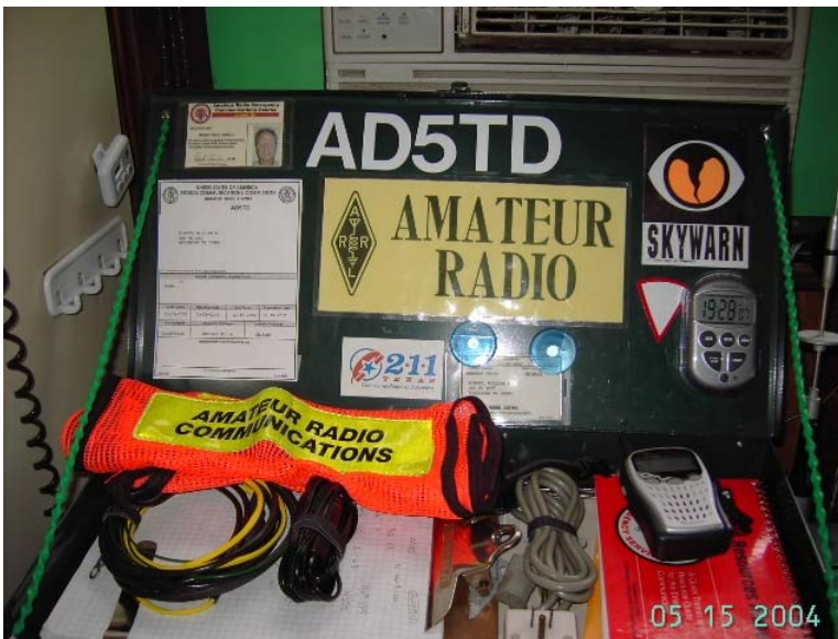
This is a view showing the top open and you can see that I have posted a copy of my License, AARECC card, timer/clock, and my call letters. Also stored on top are my vest, a roll-up J pole, power cords, weather radio, clip boards, impulse suppressor, ARRL Field Resources Manual, Mini Log Book, and Emergency Response Guidebook. There is an also a work light, and the ground plane radial for my VHF/UHF vertical antenna.
